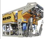
Submarine Emergency Ventilation and Decompression System (SEVDS) SEVDS provide fresh air and controlled decompression and ventilation in a DISSUB to extend life while rescue assets are being mobilized. They can be rapidly deployed to the scene and connected to the submarine by the HARDSUITTM ADS, an ROV, or conventional divers during a submarine disaster.
