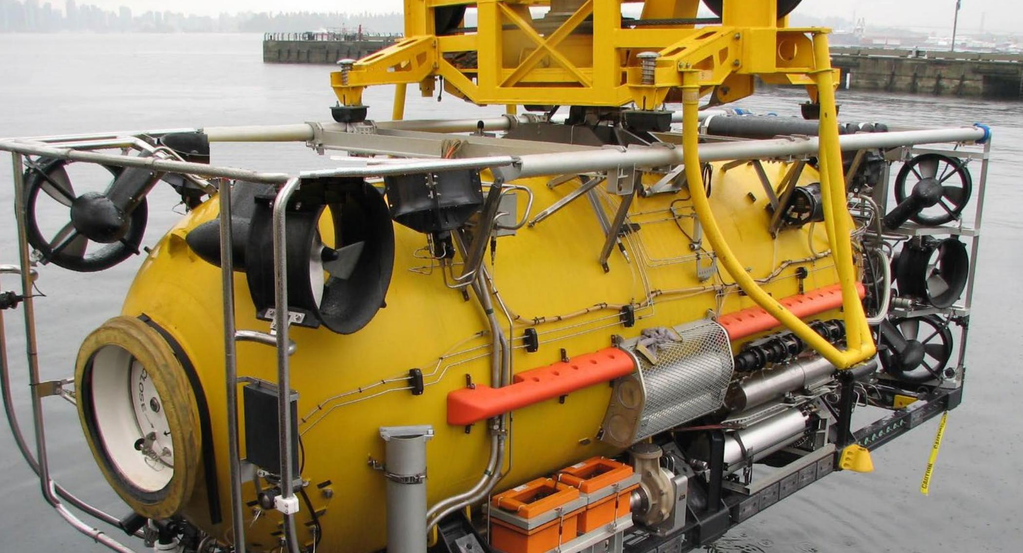
OceanWorks International's submarine rescue systems and services provide rapid response and worldwide capability for rescue of crew members from a submarine that is disabled and trapped on the seafloor (DISSUB).
